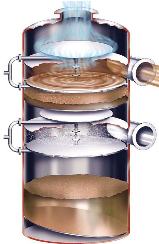
**Figure 8:** A dual chamber V-tex™ scrubber as installed at an optical fibre manufacturing plant
