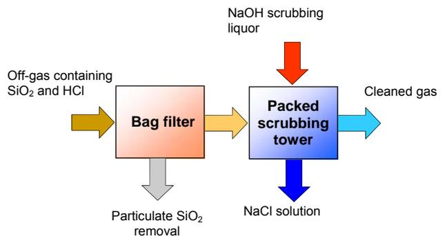
A difficulty of this approach is that in the 1<sup>st</sup> stage the dry bag filter is exposed to a corrosive environment. For the particulate to form and thus be able to be captured by the dry filter, the SiCl<sub>4</sub> must first hydrolyse in the presence of moisture which also forms highly corrosive HCl. Expensive counter measures are required to handle this aggressive environment typically involving exotic construction materials, temperature control, lagging and lime dosing.
