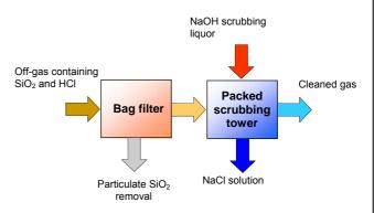
A difficulty of this approach is that in the 1<sup>st</sup> stage the dry bag filter is exposed to a corrosive environment. For the particulate to form and thus be able to be captured by the dry filter, the SiCl<sub>4</sub> must first hydrolyse in the presence of moisture which also forms highly corrosive HCI. Expensive counter measures are required to handle this aggressive environment typically involving exotic construction materials, temperature control, lagging and lime dosing.
