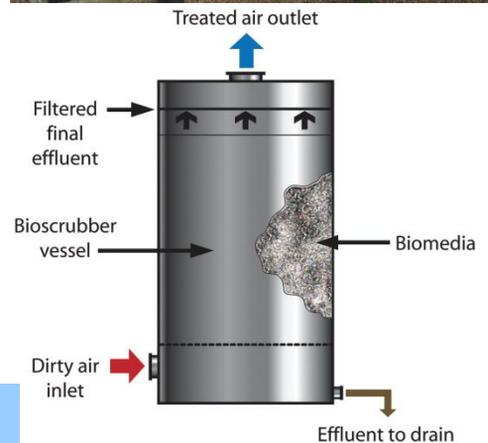
Indicative Removal of H<sub>2</sub>S, soluble VOCs and Odour for ERG Bio-trickling Filters
