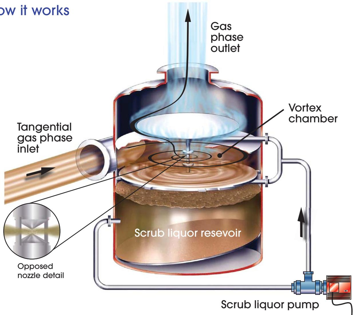
V-tex<sup>®</sup> is an innovative gas scrubber that is particularly suited to tough and challenging gas scrubbing applications where traditional scrubbing technologies cannot cope. The patented design of V-tex<sup>®</sup> harnesses the properties of a vortex to deliver exceptionally high scrubbing efficiencies within a compact footprint. It has no moving parts in contact with the process stream and no packing to foul - properties that clients across many industries value highly.
