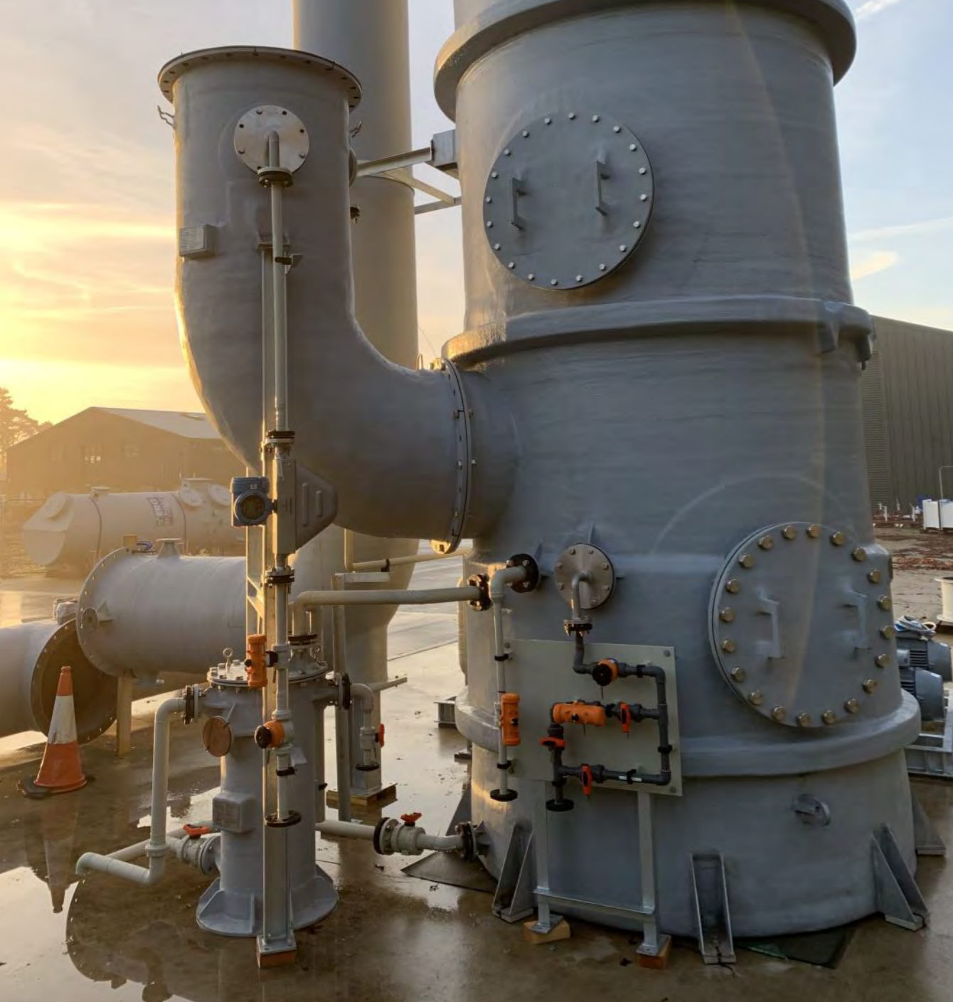
Trial assembly of the scrubber vessel and pump skid and FAT/run test at ERG's manufacturing facility in the UK
