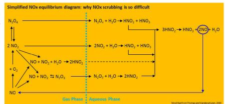
ERG's technical approach is to take the low solubility mixture of NO + NO<sub>2</sub> produced by the metallurgical processing and convert this into a more soluble gas mixture of N<sub>2</sub>O5 or HNO<sub>2</sub>.
